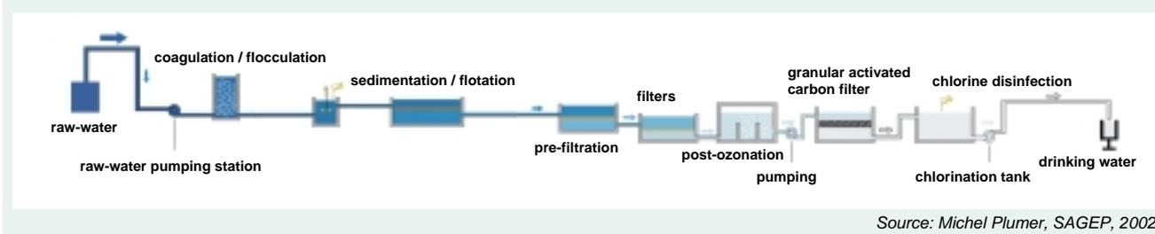
Conventional drinking water treatment, when carried out effectively (screening-prefiltration, coagulation-clarification, filtration), allows a good removal of algae and cyanobacteria.
